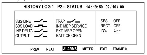
The last page includes faults. The alarm conditions that cause the History Status buffer to store and freeze data are:
